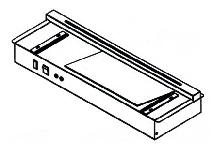
2. Adjust the material to the required position using the calibrated scales or by viewing down through the slot in the guard. Switch on the machine and heat material until flexible.
