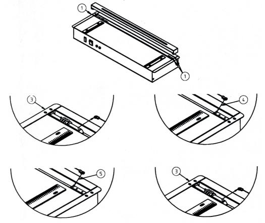
Note: during manufacture, washers may be fitted onto the wire locating pins to adjust the wire height. If fitted, these should be left in position below the heating wire terminals.
