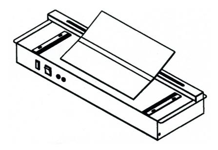
4. Fold by hand or into a cooling jig and allow to cool.
