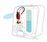
If you have waited for 5-10 minutes with the clips disconnected from the fuel cell, the fan should start rotating by itself once connected. Make sure you repeat the waiting period of 5-10 minutes after each purging. Since the reaction is slow, the fan can run for up to several hours without purging (see Experiment 3).
