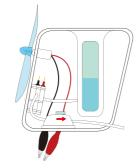
Make sure the tubing connecting the tubing with purging valve is securely connected to the fuel cell and the switch on the puraina valve is positioned at the right side close to the solution tank.
